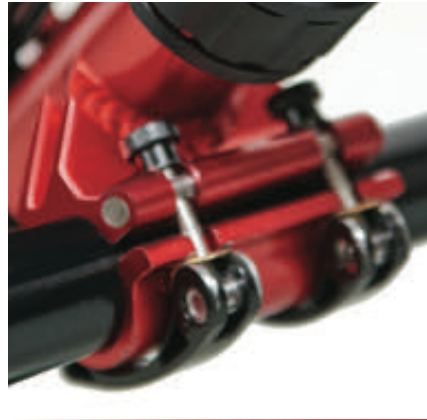
Frame easily comes apart via "Double quick release"
